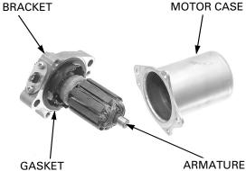
Install the motor case screws and tighten them to the specified torque.
