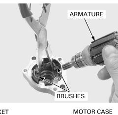
The coil may be damaged if the magnet pulls the armature against the case.
