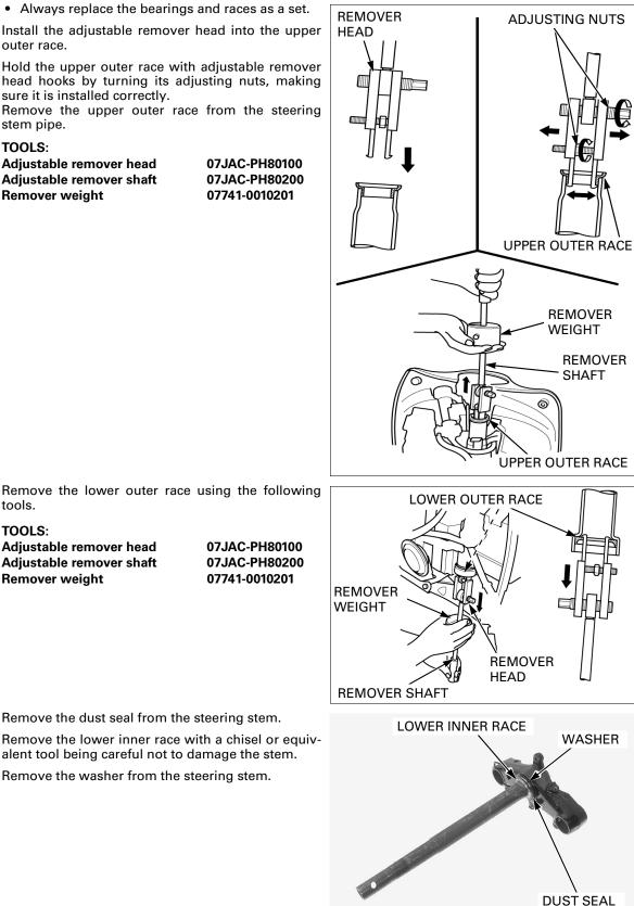
Remove the lower outer race using the following tools.
