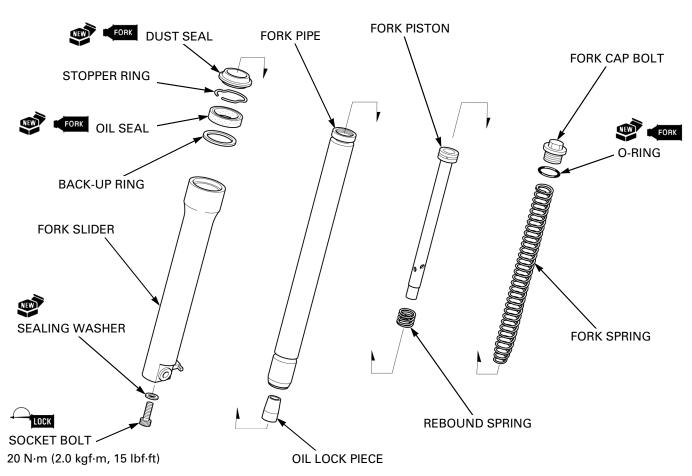
Before assembly, wash all parts with high flash point or non-flammable solvent and wipe them dry. Install the rebound spring and fork piston into the fork pipe.
