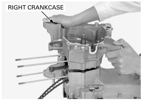
Install the crankcase bolts and tighten them in a crisscross pattern in 2 - 3 steps.
