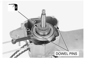
Assemble the left and right crankcase.
