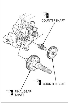
Apply sealant to the final reduction case mating surface.
