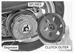
Install the washer and clutch outer nut.
