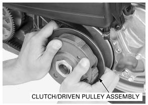
Clean any oil and grease from the clutch outer.
