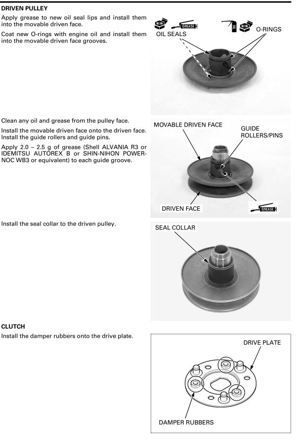
Clean any oil and grease from the pulley face.
