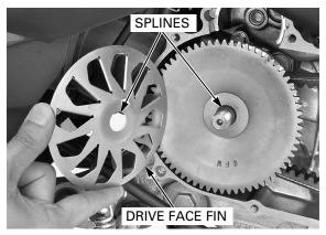
Install the drive face flange with the tapered side facing out.
