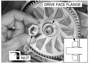
Hold the drive pulley face with the special tool and tighten the nut to the specified torque.
