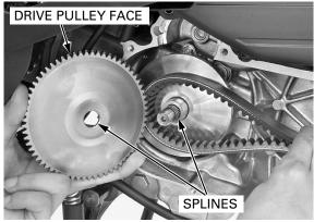
Make sure that the drive pulley face is fully seated on the drive pulley boss.
