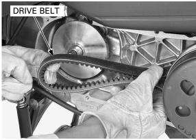
Set the drive belt onto the drive pulley boss by squeezing it to obtain the clearance between the belt and shaft.
