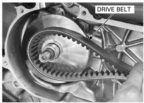
Remove the movable drive face assembly while holding the back of the face (ramp plate) and drive face boss.
