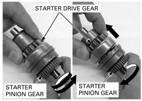
Check the pinion gear teeth and shaft for wear or damage.
