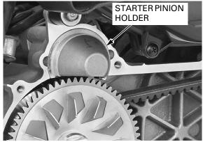
Remove the starter pinion.
