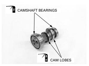
Install the camshaft into the camshaft holder. Set the stopper plate and hold the camshaft.
