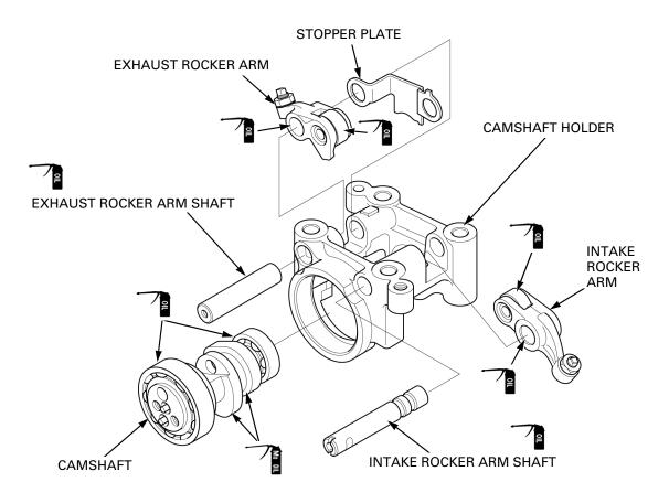
Apply engine oil to the camshaft bearings. Apply molybdenum oil solution to the cam lobes.
