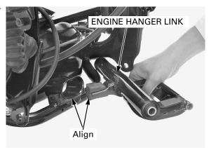
Install the engine hanger link pivot bolt (frame side) from the right side of the frame.
