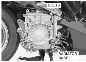
Install the radiator base and bolts. Install the following:
