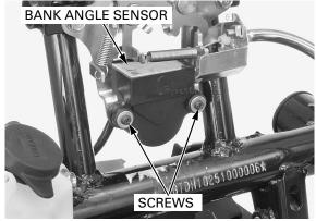
If you perform this test, turn the ignition switch "OFF", then turn the ignition switch "ON". Place the bank angle sensor in normal position as shown, and turn the ignition switch "ON". The bank angle sensor is normal if the engine stop relay clicks, which indicates that circuit is closed.
