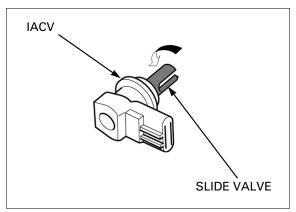
Install the IACV by aligning the pin with the slide valve slot.
