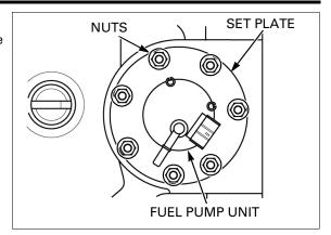
Remove the packing from the fuel pump unit.
