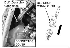
If the ECM has no stored failure code, the MIL will illuminate, when you turn the ignition switch "ON".
