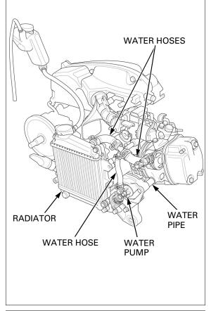
Check the radiator air passage for clogs or damage. Straighten bent fins with a small, flat blade screwdriver and remove insects, mud or other obstructions with compressed air or low pressure water. Replace the radiator if the air flow is restricted over more than 20% of the radiating surface.
