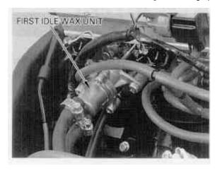
When the engine coolant temperature is low, the wax unit shaft is pulled into the wax body by the force of the return spring in the wax unit.
