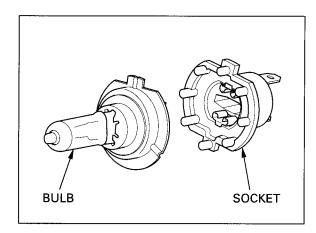
Install the headlight bulb/socket aligning its tabs with the groove in the headlight unit.
