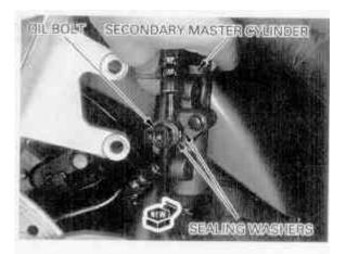
Place the secondary master cylinder onto the fork leg, then tighten the new mounting bolts.
