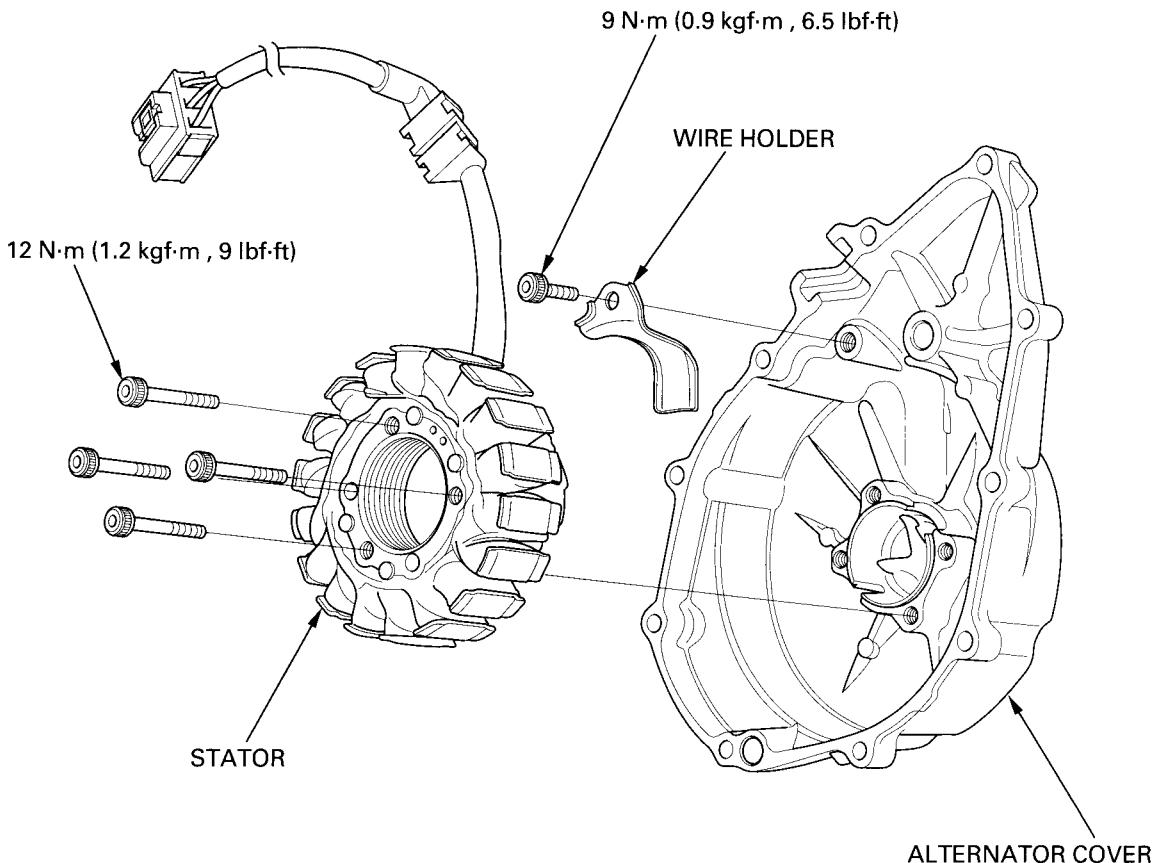
Install the stator into the alternator cover.
