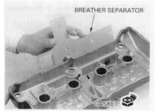
Apply a locking agent to the crankcase breather separator mounting bolt threads.
