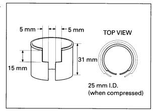
Remove the valve spring cotters using the special tools as shown.
