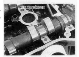
Install the camshaft holders and tighten the bolts in a crisscross pattern in 2-3 steps.
