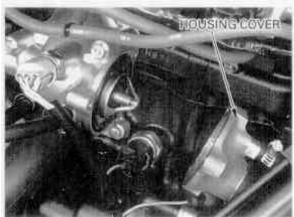
Install and tighten the housing cover bolts.
