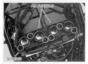
Release the air cleaner housing from the ram ducts.
