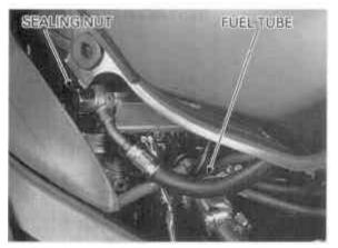
Disconnect the fuel return tube at the throttle body.
