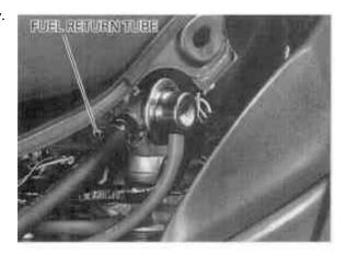
Pull the fuel tank backward and release the front bracket from the frame.
