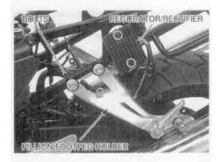
Install the right pillion footpeg holder onto the seat rail, tighten the mounting bolts to the specified torque.
