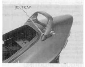
Remove the two socket bolts. Remove the setting bolts, collars and rear grip.
