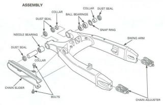
Press the needle bearing into the pivot with the marked side facing out. Pack the new needle bearing with grease.
