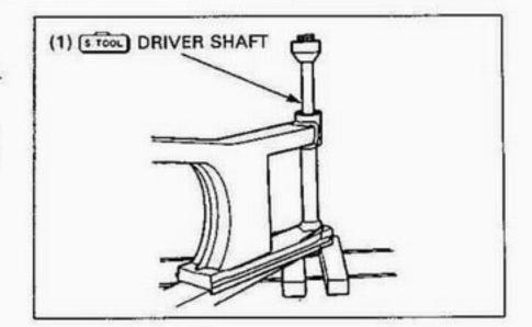
Set the needle bearing remover onto the left pivot bearing (needle bearing) as shown.
