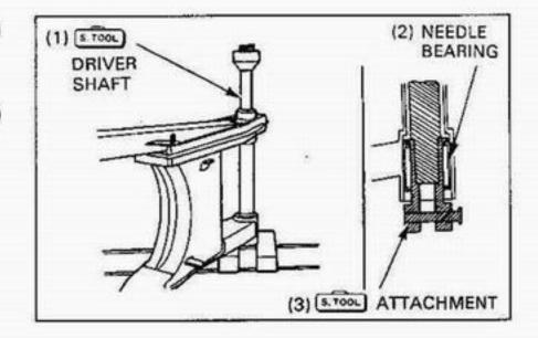
Press the needle bearing into the swingarm with the marked side facing out.
