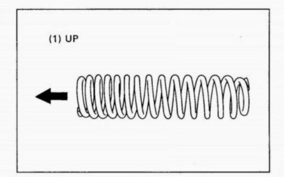
Install the special tools and compress the shock spring. Install the lower seat securely.
