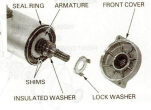
Install the shims properly as noted during removal. Install the seal ring on the motor case. Install the shims on the armature shaft.
