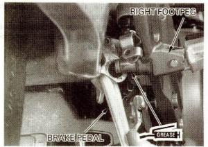
Install the washer and secure the brake pedal with a snap ring.
