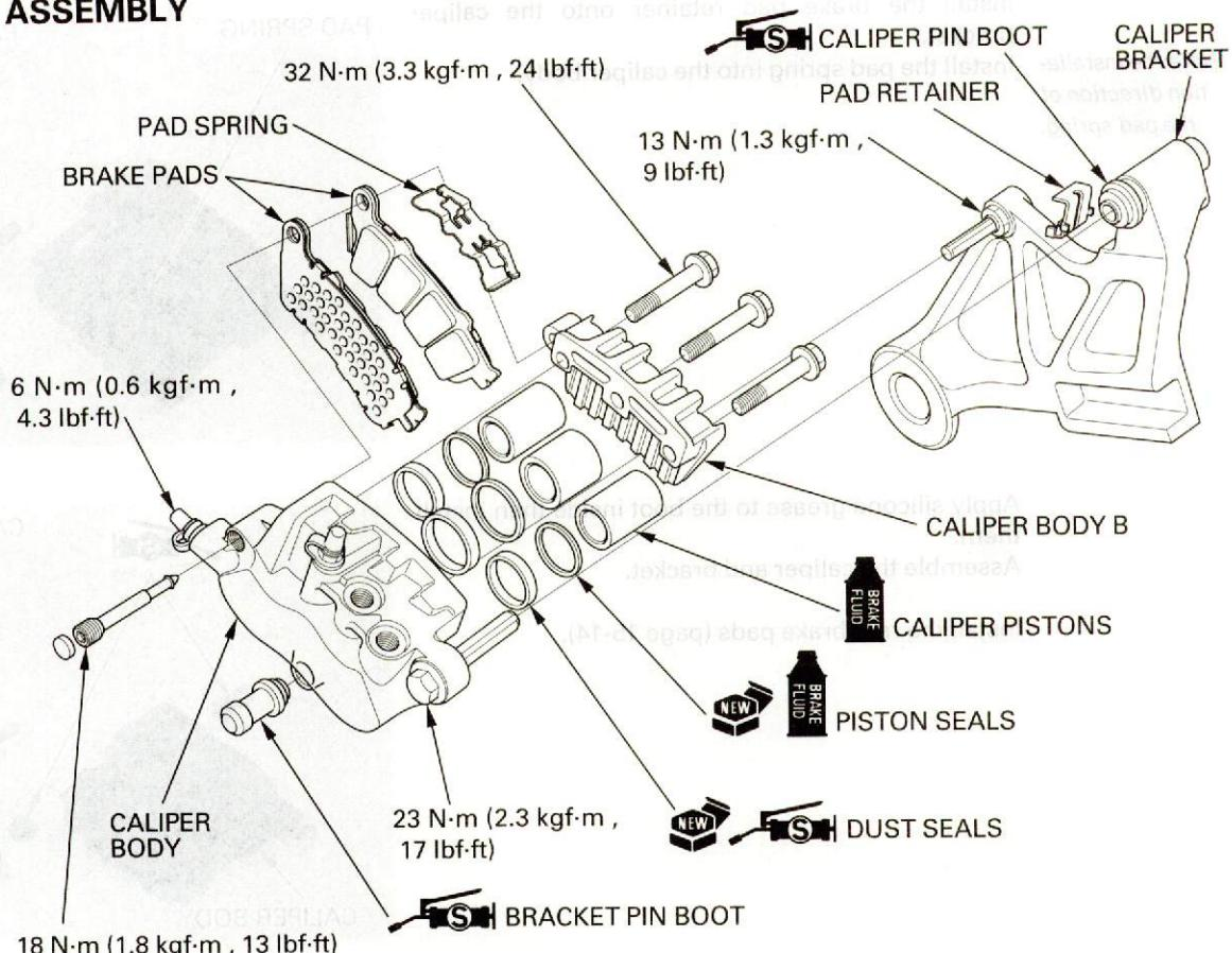
Coat the new piston seals with clean brake fluid.
