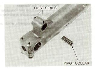
Press out the pivot bearings using the special tool.
