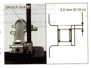
Apply grease to the new dust seal lips. Install the dust seals and pivot collar.
