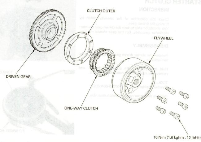
Apply oil to the starter one-way clutch.
