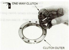
Install the starter one-way clutch assembly onto the flywheel.
