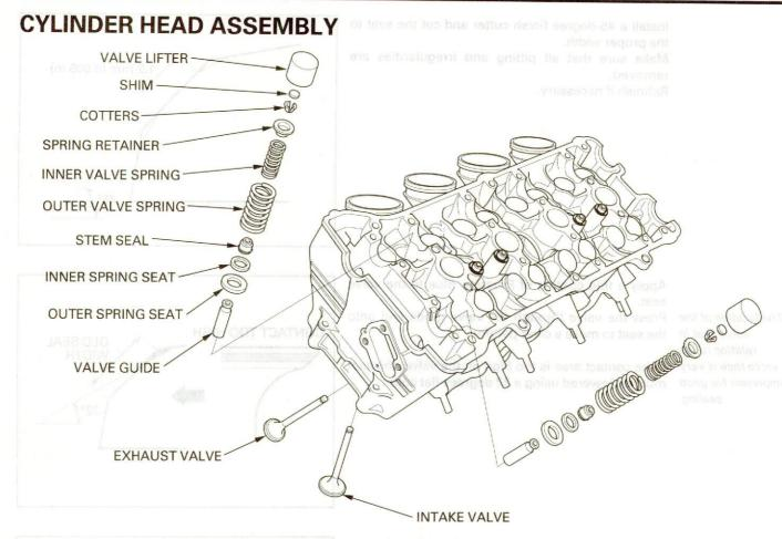
Clean the cylinder head assembly with solvent and blow through all oil passages with compressed air.
