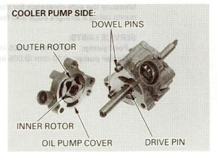
Install and tighten the assembly bolt to the specified torque.
