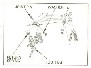
Push the new retaining clip into the joint pin hole. Turn the retaining clip with the joint pin, then hook the clip end into the V-cut groove of the footpeg holder.
