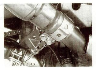
Loosen the muffler front mounting nut.
